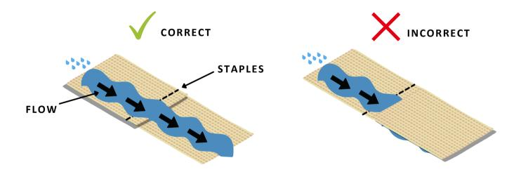
**STEP 4:** Roll the remainder of the Erosion Control Blanket out to cover the installation area. If using multiple rolls, allow a 12" overlap, layering the overlapping blanket edges so that water flow is not obstructed. Secure the overlapped seams with staples at 5" intervals.
