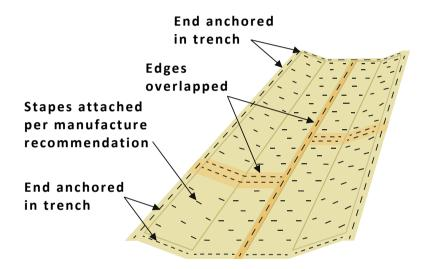
**STEP 6:** Secure the remainder of the blanket at staggered intervals, following the pattern guideline below for your site's flow rate and conditions.
